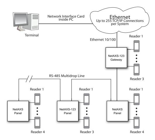
This configuration supports a total of 31 NetAXS and NetAXS-123 panels per Multidrop line.
